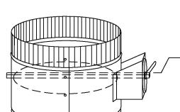
Damper with nylon bushings, 3/8" continuous rod and locking steel regulator on 2" stand off.
