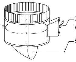
Damper with nylon bushings and 1/4" locking steel regulator on 2" stand off.
