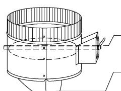
Damper with nylon bushings, 3/8" continuous rod and locking steel regulator on 2" stand off.
