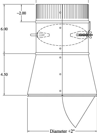
PART #: 505DX(Size) **DESCRIPTION:** Conical Metal Spin In Starting Collar
