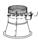
Damper with nylon bushings, 3/8" continuous rod and locking steel regulator on 2" stand off.
