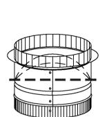
10", 12" and 14" diameters available Damper rest Sealant tape
