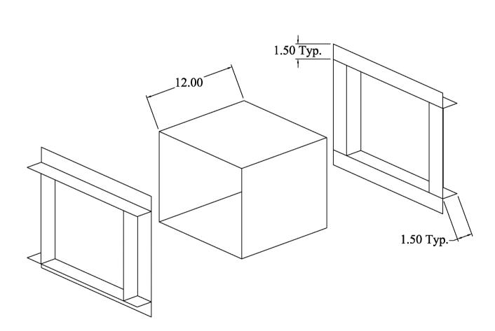
PART #: MP-FDA(Size) DESCRIPTION: Fire damper sleeve and retaining angle set
