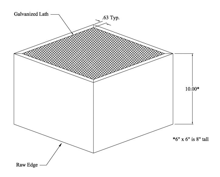
PART #: V-CAV(Size) DESCRIPTION: Combustion Air Vent
