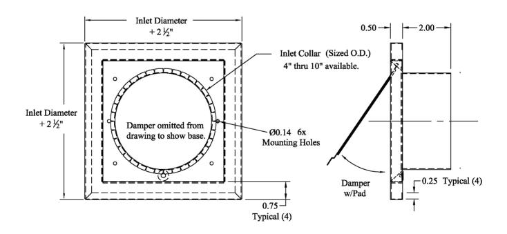
PART #: V-SBLV(Size)PCWP DESCRIPTION: Powder coated flush mount wall vent
